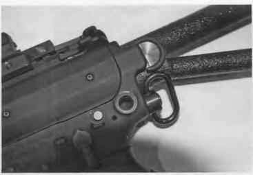
This close-up shows the PDW's folding stock mechanism and sling mounts.
